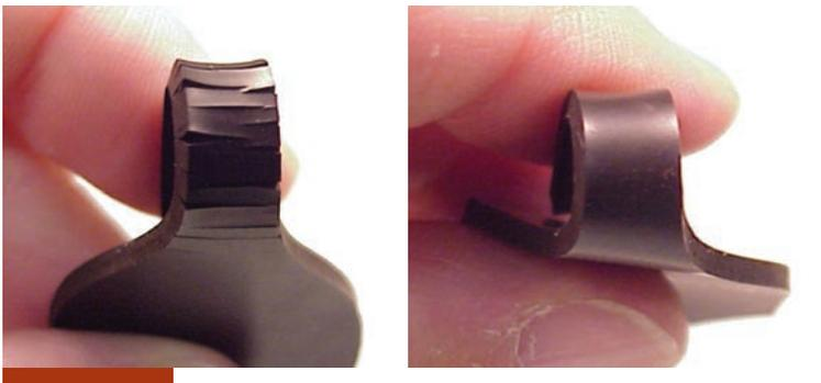
**THE FLUOROCARBON** elastomer specimen that became brittle with visible cracks vs. no cracks. EXXONMOBIL
