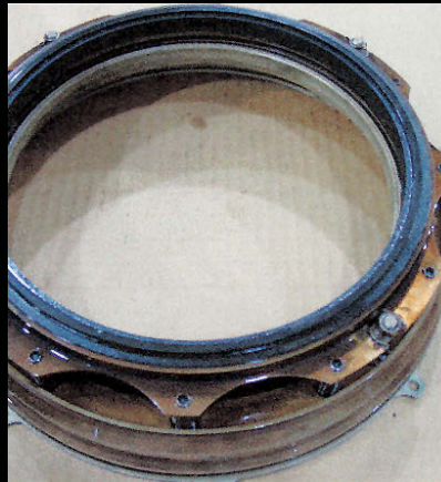
No. 3 carbon seal. Very good condition. Negligible light varnish deposits.
