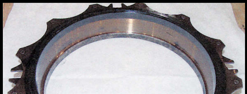
No. 4 carbon seal. Very good condition. Negligible light varnish deposits.
