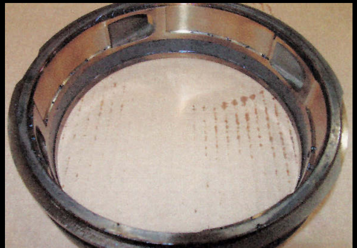
Oil slinger. Very good condition. No sludge. Negligible light varnish deposits.
