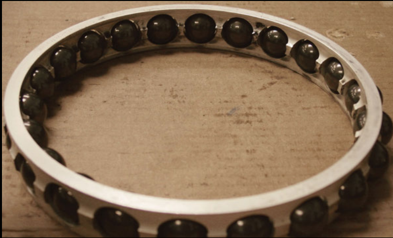
Mobil Jet™ Oil II. Excellent condition. Negligible deposits.
