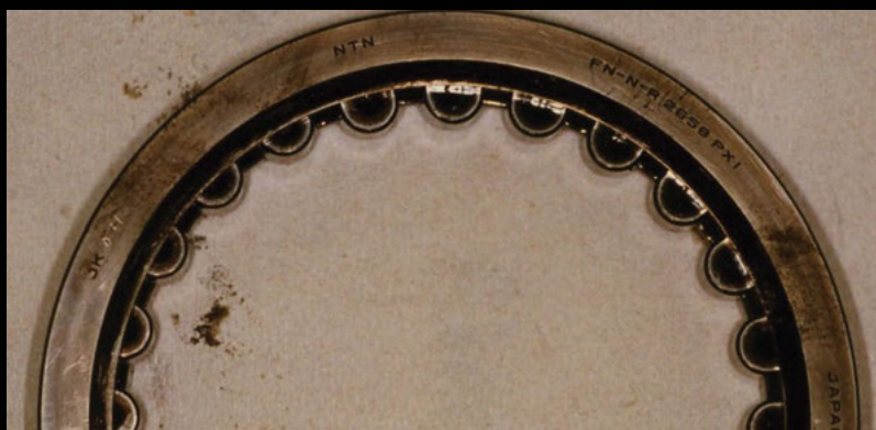
Competitive Type II oil. Varnish and black oil deposits.
