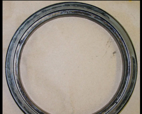
Mobil Jet Oil II. Very good condition. Negligible deposits.
