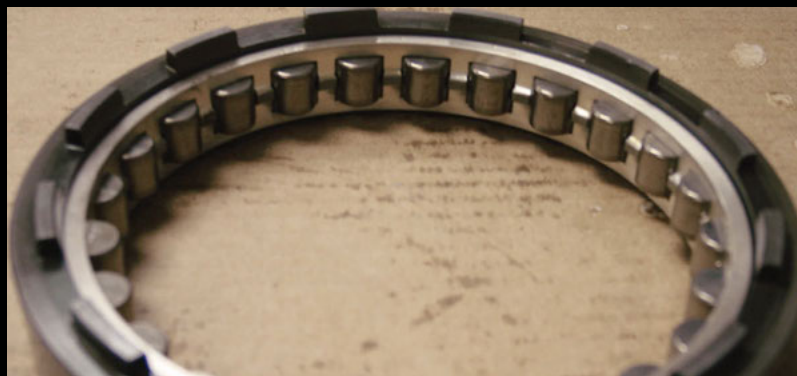
Mobil Jet Oil II. Very good condition. Negligible deposits.
