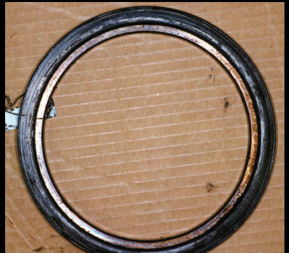
Competitive Type II oil. Varnish and black oil deposits.
