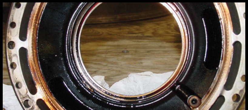
Competitive HTS oil. Very thin black varnish and carbon deposits.
