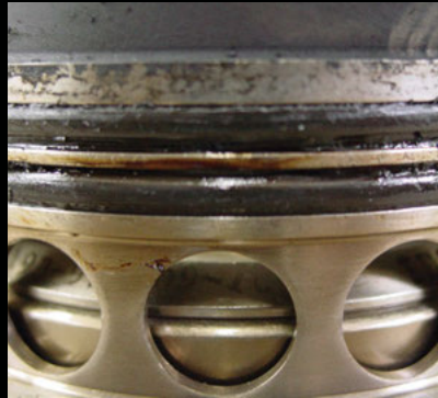
Mobil Jet Oil II. O-rings in grooves in very good condition and sealing.
