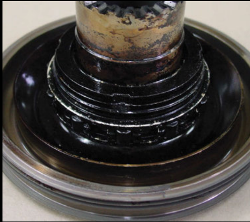
Mobil Jet™ Oil II. Thin black varnish and carbon deposits.
