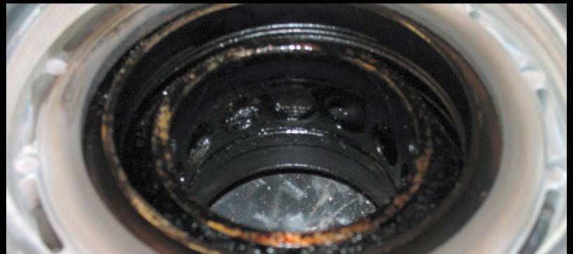
Mobil Jet Oil II. Thin black varnish and carbon deposits.
