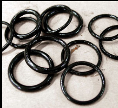
Mobil Jet Oil II. O-rings in very good condition, pliable.
