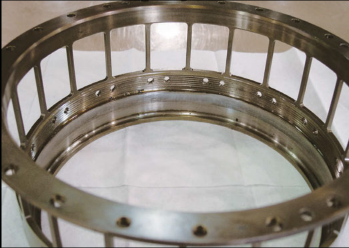
No. 4 bearing housing. Excellent condition. Light varnish deposits.
