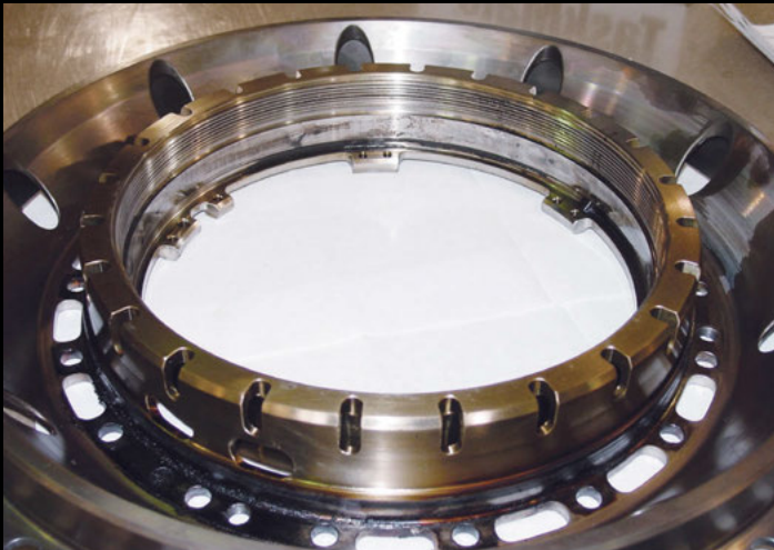
No. 5 bearing/seal housing. Excellent condition. Light varnish deposits.
