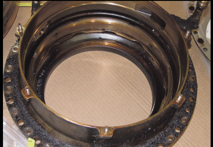
No. 6 bearing housing - turbine rear frame. Excellent condition. Light varnish deposits.
