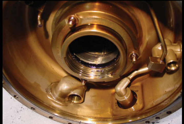
No. 7 bearing/seal housing. Excellent condition. Very light varnish deposits. Carbon seal in very good condition.
