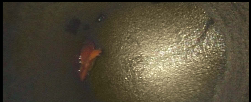
Scavenge oil tube. Negligible deposits. No reduction in area inside. The small piece of carbon and non-metallic flake migrated from another area of the engine.
