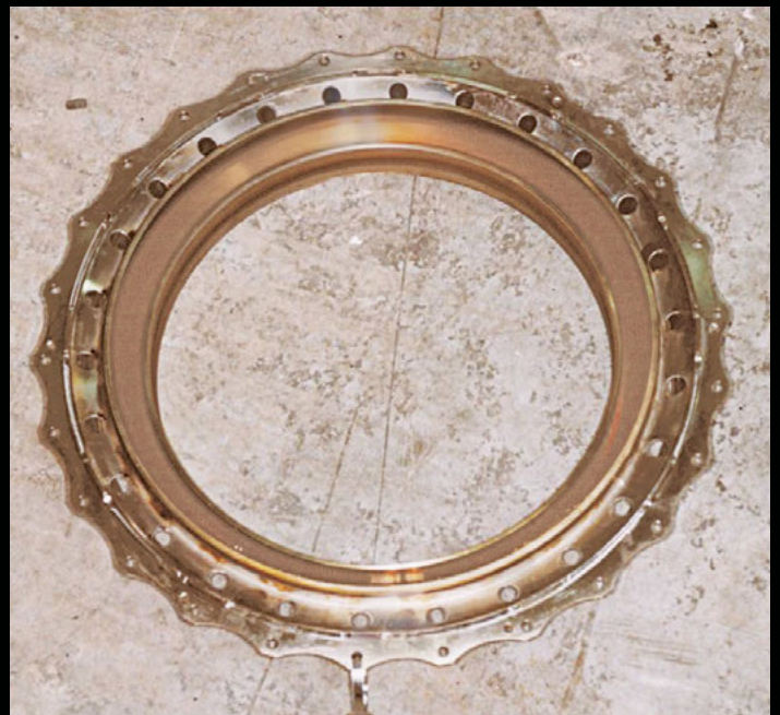
No. 5 stationary oil seal. Very good condition. Negligible deposits.
